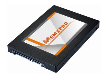
The MemxPro 2.5" SSD-P series feature Power Plus for creating power backups during unexpected power failure. Power Plus with firmware control and capacitor design provides enough power hold-up time for all data in the DRAM buffers to be totally written back to the NAND flash, ensuring total user data integrity.
